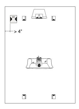
U1 Subwoofer System: The U1 subwoofer enclosure is a dual, side-firing design. If the U1 is going to be located in a corner or against a wall, we recommend that you keep the face with the grille at least 4" from any boundary to obtain optimum performance.
